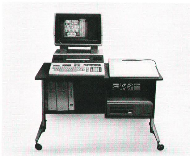
Fig. 1. The PIGLET station provides a compact interactive graphics design system for IC and printed-circuit layouts, schematic drawings, plant layout, and illustrations. It supports the same symbolic design capability that is available with IGS.
