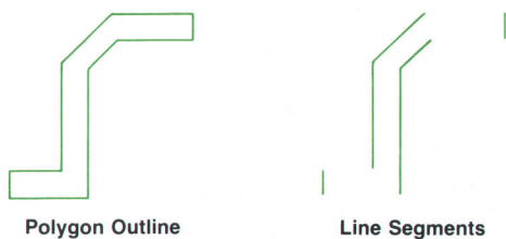
Fig. 6. DRC data representation. Polygon outlines are represented using an efficient line-segment method.
